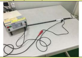
Dielectric Withstanding Voltage Test
